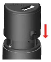
Align the housing to the base plate, slide the housing onto the base plate
