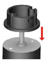
Align the base plate to the motor shaft by using the centering gauge
